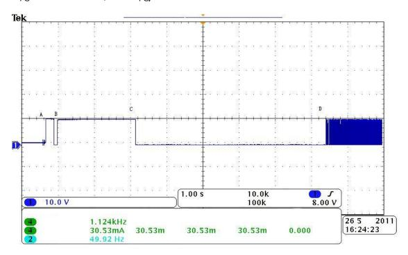
The signal waveform when white line then pulled to 10V with 47K resistor.
