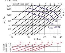
Effect of distance X and open rows of holes to the noise level at different connections
